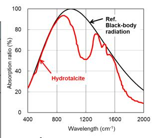
[Heat retention performance (infrared absorption rate)]
